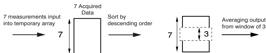
Figure 28. MAV Filter Operation (Patent Pending)
